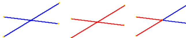
Figure 3-22: Divide independent lines/arcs by intersection
