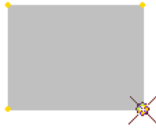
Figure 3-15: Snap to the corner of a rectangle when create a new line
